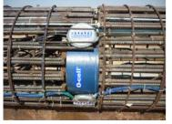
Pile reinforcing cage with O-cell instrumentation
